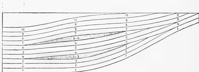
FIG. 131. Diagram illustrating the changes in stratification due to subaqueous gliding. In the shore section strata are eliminated, while farther out duplication occurs. (After Heim.)
